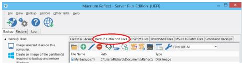
In this instance, there is one saved XML definitions file MyBackup.xm/which contains the configuration required to back up the C drive.
