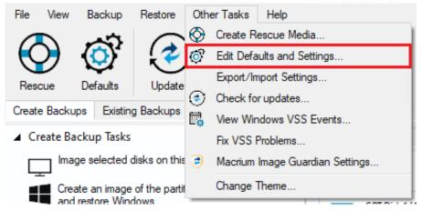
Windows contains a Network Credentials cache that enables network authentication details (User name and password) to be saved and re-used to logon automatically. However, scheduled tasks are run in Windows 'batch mode' and do not have access to saved credentials. Because of this, you must enter network login details in the Macrium Reflect defaults to enable scheduled tasks to access and write to password-protected network shares.
