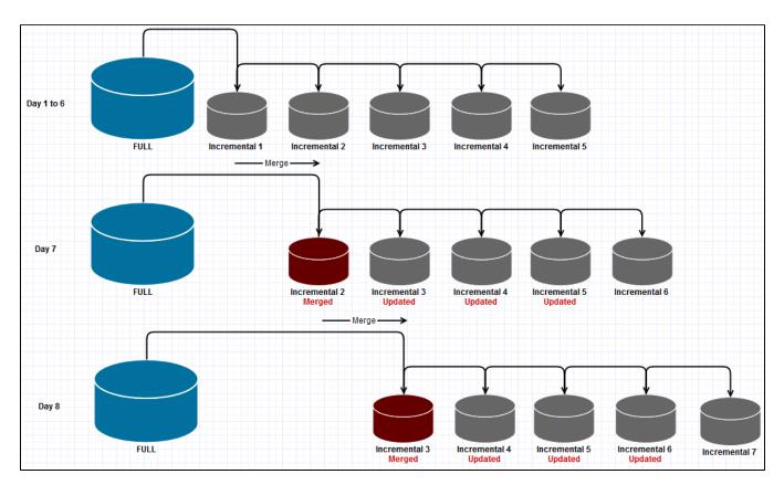
In this example, when the 6th Incremental is created, the first Incremental is merged with the second and existing Incremental images 3 - 5 are updated to indicated that Incremental 1 is no-longer in the backup chain by modifying the file index. This process is repeated for each subsequent Incremental that is run.
