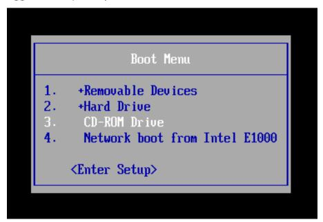
Chose CD-ROM drive or a Removable USB device based on the choice of Rescue Media you've built and press Enter to load the Rescue Media.
