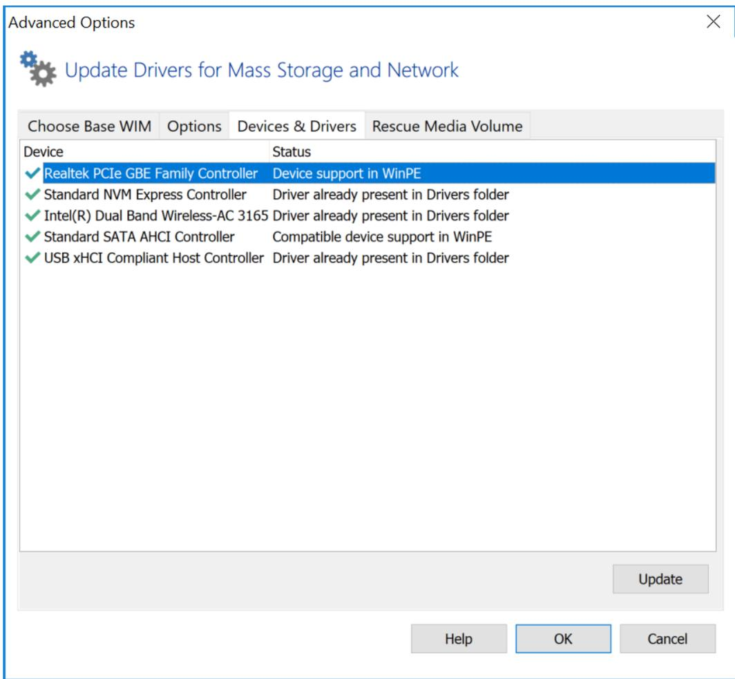
Mass Storage and Network devices will be listed showing the current state of driver support. Drivers can be added for devices missing driver support as well as updating drivers previously added to the rescue media.
