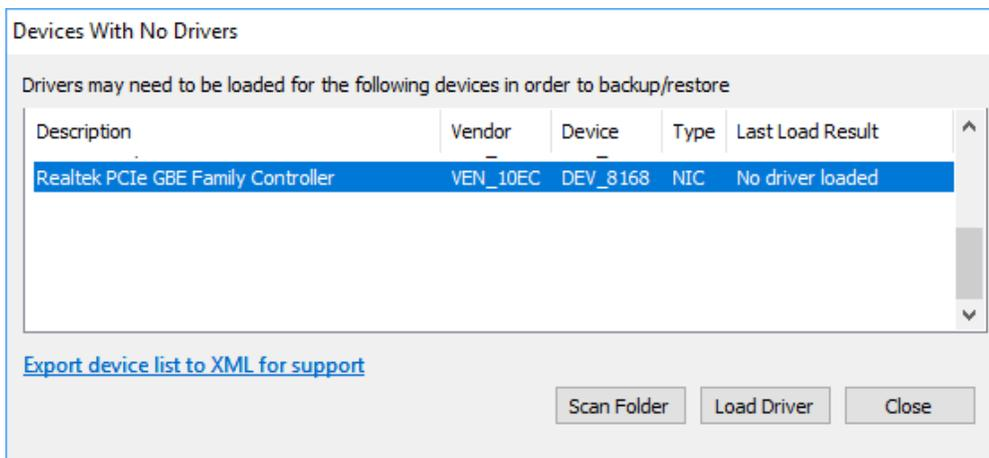
a list of devices which are currently unsupported will be shown. Drivers can be loaded using two methods:
